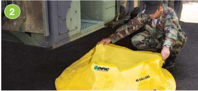
Step 2: Position pool underneath spill source.
